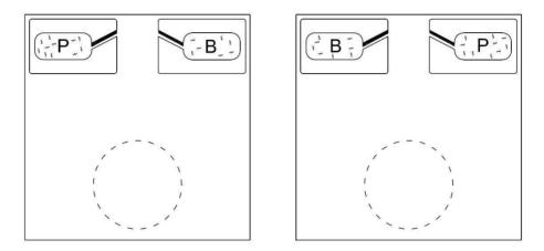
Fig. 1. Scheme of laboratory experiment. In square Petri dishes  $(10.2 \text{ cm} \times 10.2 \text{ cm} \times 1.9 \text{ cm})$  two artificial nest chambers were placed – one filled with fresh pine shavings (P), and one with fresh beech shavings (B). Ants were released close to the opposite edge of the Petri dish (an area marked with a dotted line)
