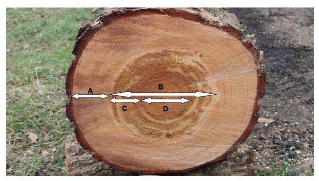
Fig. 1. The Scots pine's cross section on the 3,20 m height. By arrows there were tagged: A – uninfected sapwood, B – infected heartwood, C – early decay, D – late decay. Area infected by the early decay is covered with characteristic darker crescent pattern – the effect of lignin decomposition.
