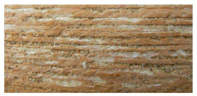
Fig. 2. The Scots pine's longitudinal section on the 3.5 m height. View characteristic for non selective delignification: dark color of lignin on which variform lumens filled with white cellulose were visible.
